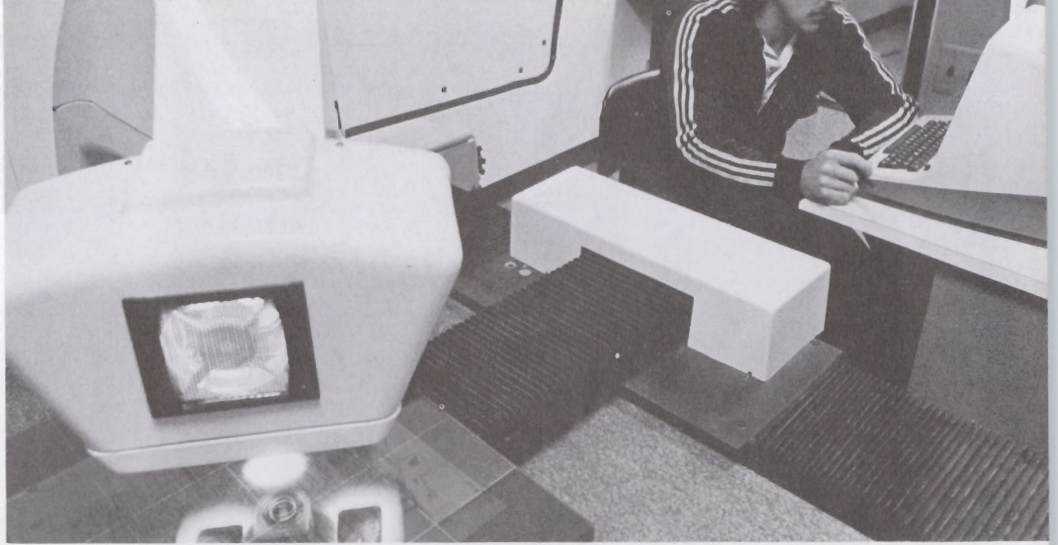
A numeric control programmer, under the direction of Steve Parish, locates the places on a circuit design where holes are to be drilled on the PC board, and records a program on tape to guide the drilling machine.
